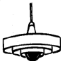
Concentric ring unit with incandescent silvered-bowl lamp
