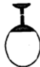
Pendant diffusing sphere with incandescent lamp
