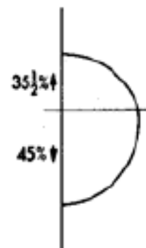
Pendant diffusing sphere with incandescent lamp
